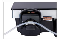
7 PIEZOSURGERY<sup>®</sup> Insert irrigation tube into peristaltic pump
